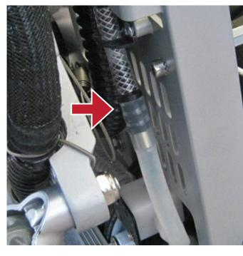
**3** Check if the solution reduction fitting is dirty/clogged.
