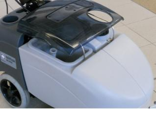
18. Park the machine with the recovery tank cover open.
