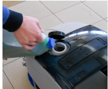
3. Always follow the dilution instructions on the label of the chemical product used to prepare the solution. The solution temperature must not exceed 40°C and be none foaming
