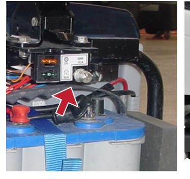
1 Check if the fuse has triggered.
