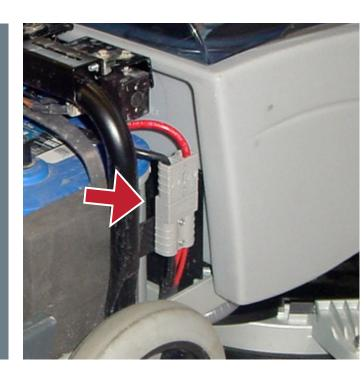
Check if the power cable is correctly 2 Check if the battery is charged.
