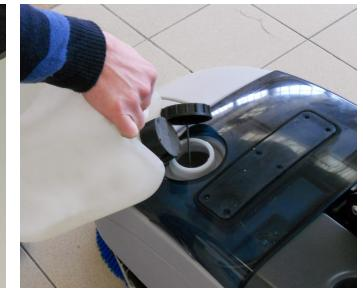
1. Disconnect the battery charger cable 2. Fill the tank with a solution suitable for the work to be performed. from the electrical main.
